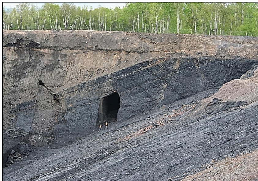
Figure 5.2. An opencast coal mine in a thick dipping coal seam, revealing an old deep mining adit. Foord seam in the Carboniferous Stellarton Formation, Stellarton, Nova Scotia, Canada
