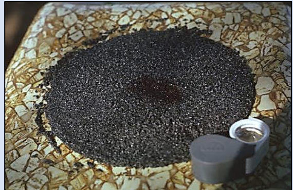
Heavy mineral jig concentrate in the field
