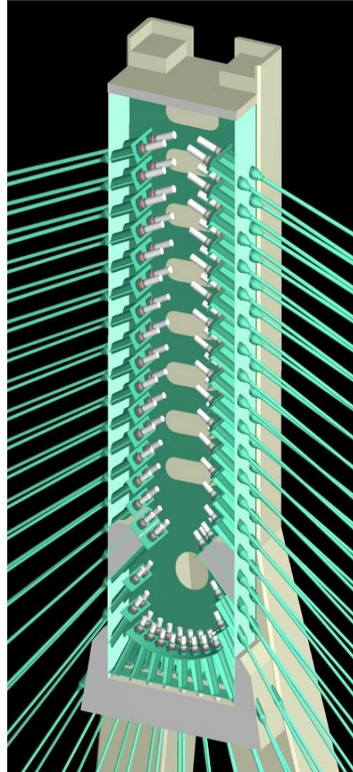
High strength concrete (C60/75) pylon legs support the steel pylon head anchorage device
