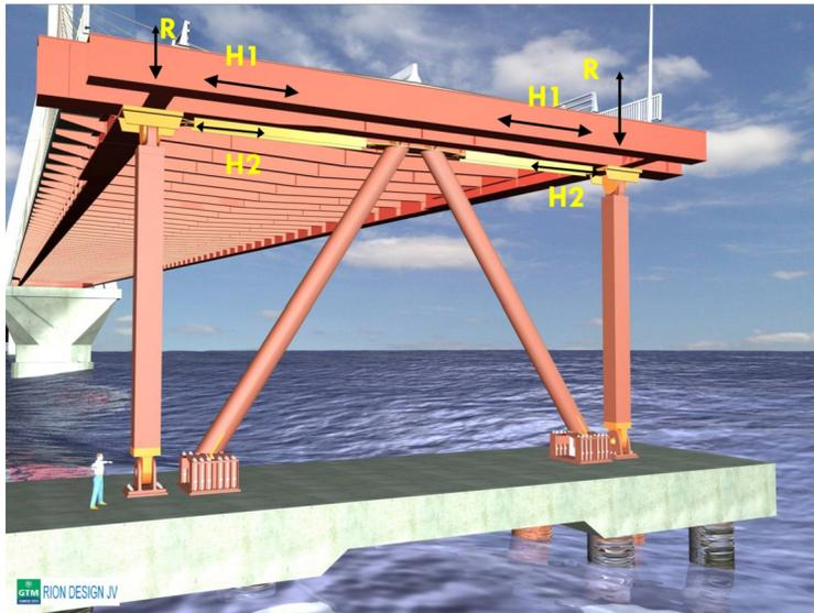
Rotating frame: steel device supporting deck edges and restraining lateral movements during normal operation conditions
