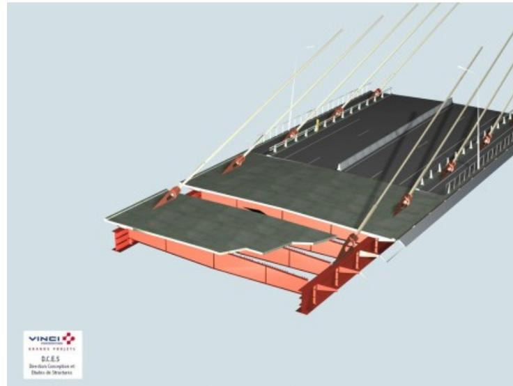
Deck: Continuous composite structure assembled with 12-m segments with total width 27m and fully suspended from pylon head
