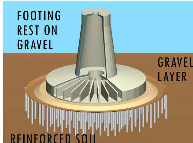
Weak soil was reinforced with steel inclusions (steel pipes 2m diameter)
