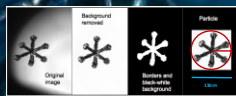
FIG. 4. Snow crystal classification system of Magono-Lee. Left: Original image. Right: Image after background removal and particle segmentation.
