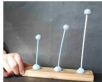
Photo 2: Blutak™ 'buildings', secured to a wooden base by more Blutak™. The middle 'building' is swaying as the base is moved backwards and forwards on the table top. (Photo: Peter Kennerly)
