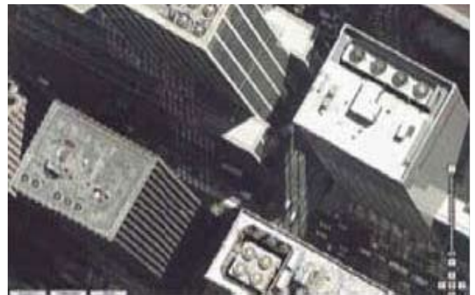
Figure 3b: Rooftop building units in New York (from Google Earth). There are in NYC alone, 6000 high rise, and 10 000 medium rise (approx 10 stories) buildings that are all pumping out such concentrated heat, not to mention all the individual window air conditioners.
