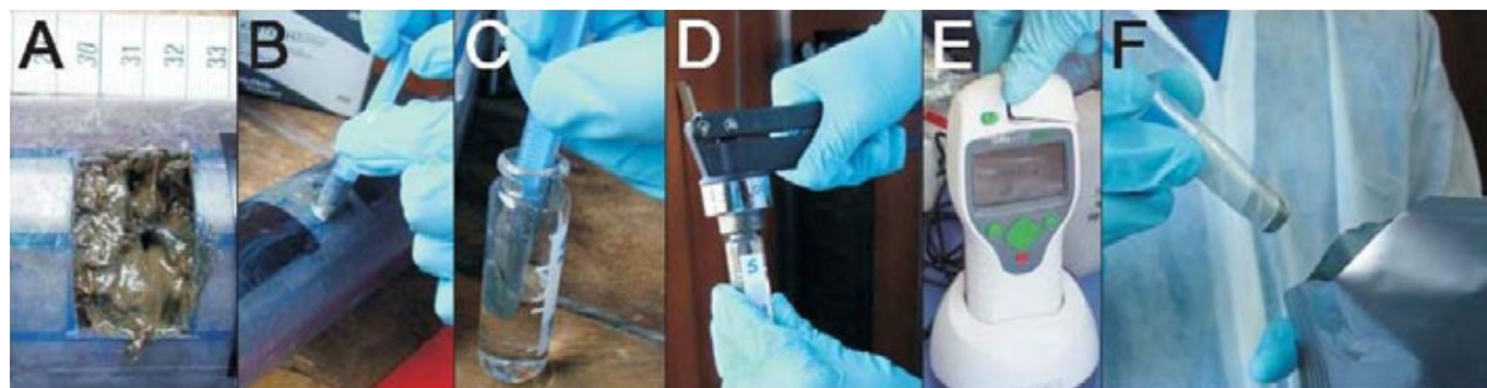
Figure 3. [A] Window cut for sampling; [B-D] sampling for methane headspace determinations; [E] preparation of the sample for in situ ATP measurements: sample is mixed with deionized water prior to centrifugation, then tested with the Uni-Lite ® NG water tester (shown); and [F] storage of the remaining sediment for cell culture. Refer to text for details. Credits: Aurèle Vuillemin.
