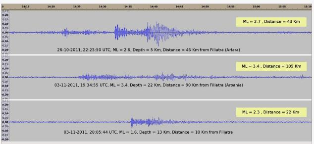
Fig. 4: Earthquake signals recorded with our homemade seismograph. The values in the yellow boxes were calculated from the homemade seismograph data, while the values under the signals are from the reports of the Institute of Geodynamics of National Observatory of Athens. ML stands for local magnitude (ML) on the Richter scale. (Credit: Panteleimon Bazanos)
