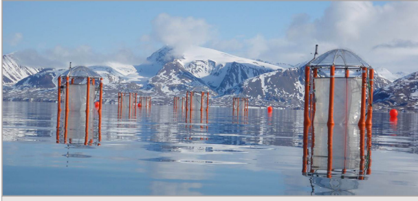
Fig. 2: Mesocosm facilities developed at the GEOMAR | Helmholtz Centre for Ocean Research Kiel, used during the second EPOCA campaign in Svalbard, summer 2010.
