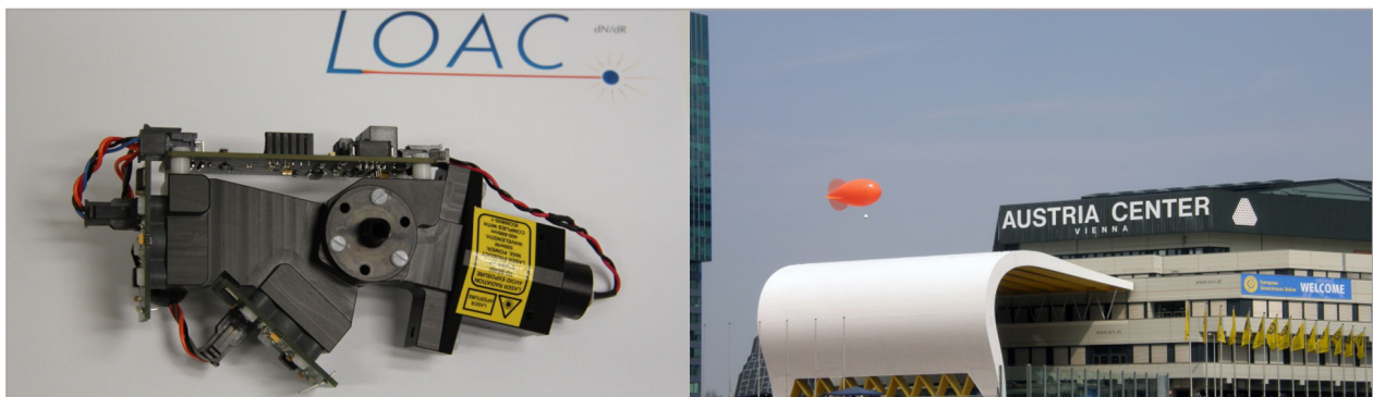
Figure 1. Left: LOAC optical chamber and electronics. Right: LOAC balloon deployment at the EGU 2013 – the aerosol counter is in the small white box under the balloon. (Credit: F. Dulac)
