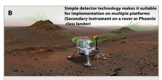
Exploring the geology of Mars with muon radiography – operational concept option B: the instrument is mounted on a small Phoenix class lander observing multiple targets during the life of the mission. (Image and caption from Kedar et al., 2013)
