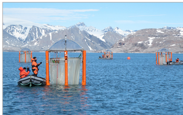
Researchers check the 'mesocosms', eight-metre long floatation frames carrying plastic bags with a capacity of 50 cubic metres, deployed for a five-week long field study on ocean acidification conducted in the Kongsfjord off the Arctic archipelago of Svalbard. (Credit: Ulf Riebesell/GEOMAR)
